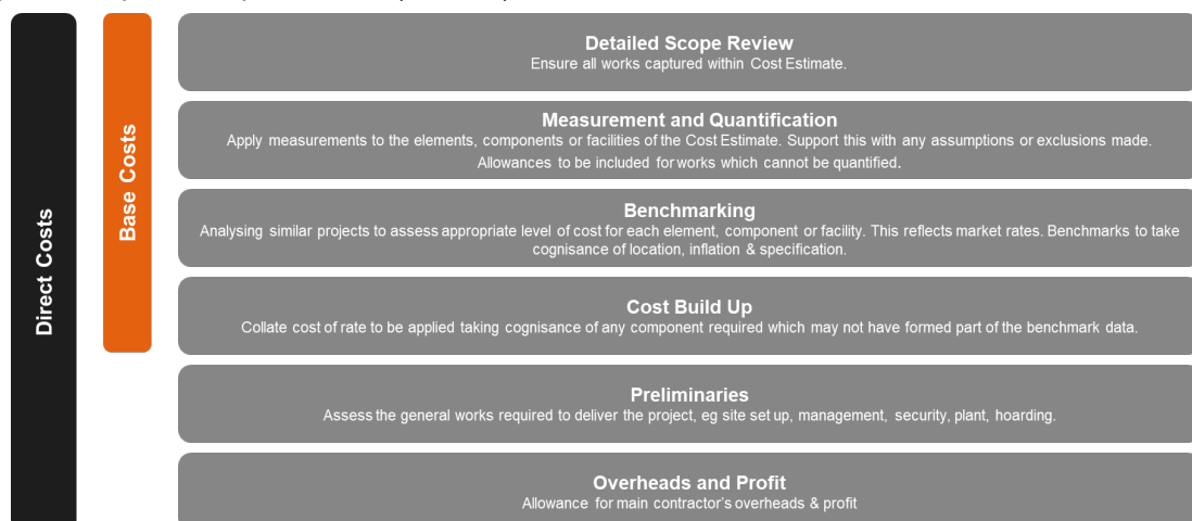
Figure 19 Approach to Cost Estimating, Direct Costs
